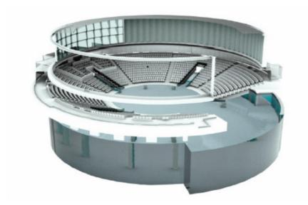
The 270-degree theater-in-the-round has a central stage with a diameter of approximately 656 feet, surrounded by sloped seating on three sides for as many as 2,000 theatre patrons.
